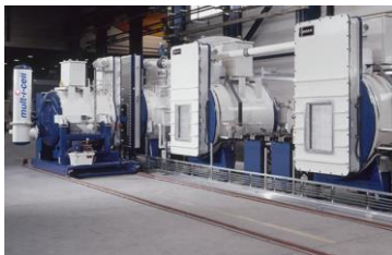
Multi chamber furnaces: Argos etc.
