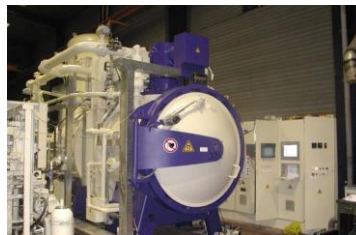
Two chamber furnaces with high pressure gas quenching
