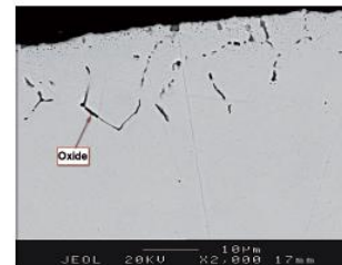
Figure 8.4.27 Internal oxidation. Backscatter SEM image of a polished sample.
