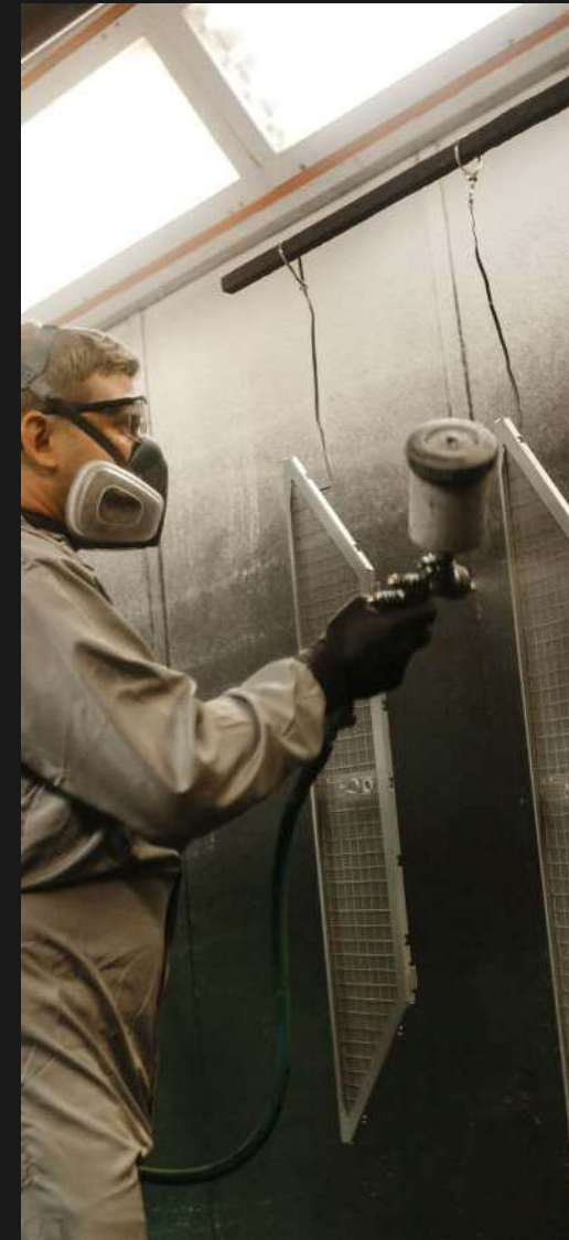
Painting, including full pre-treatment self-adhesive film coating.
