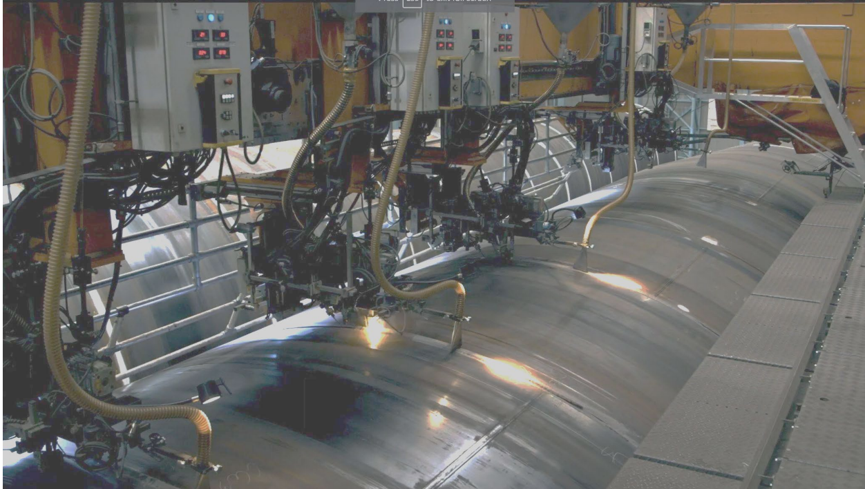
Figure 2.1: Automated Welding in a Monopile Factory, SIF Group (2020)
