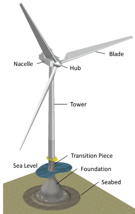
Figure I.1: Offshore wind turbine supported by a Gravity-Based Foundation, courtesy of Sigurd Ramslie, Seatower AS.
