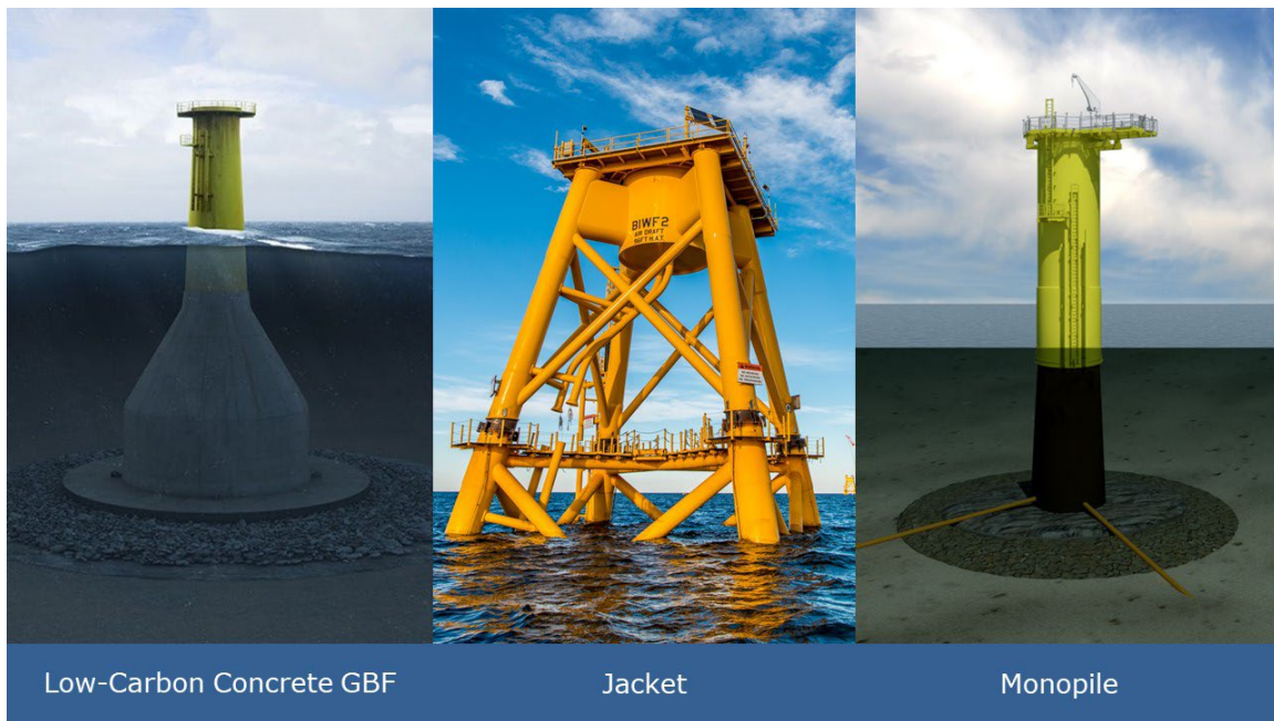
Figure I.2. Offshore wind foundations: Low-Carbon Concrete Gravity-Based; Jacket; Monopile. (image credits: GBF—Seatower 6 , AS; Jacket—offshoreWIND.biz 7 ; Monopile—Ramboll 8 )
