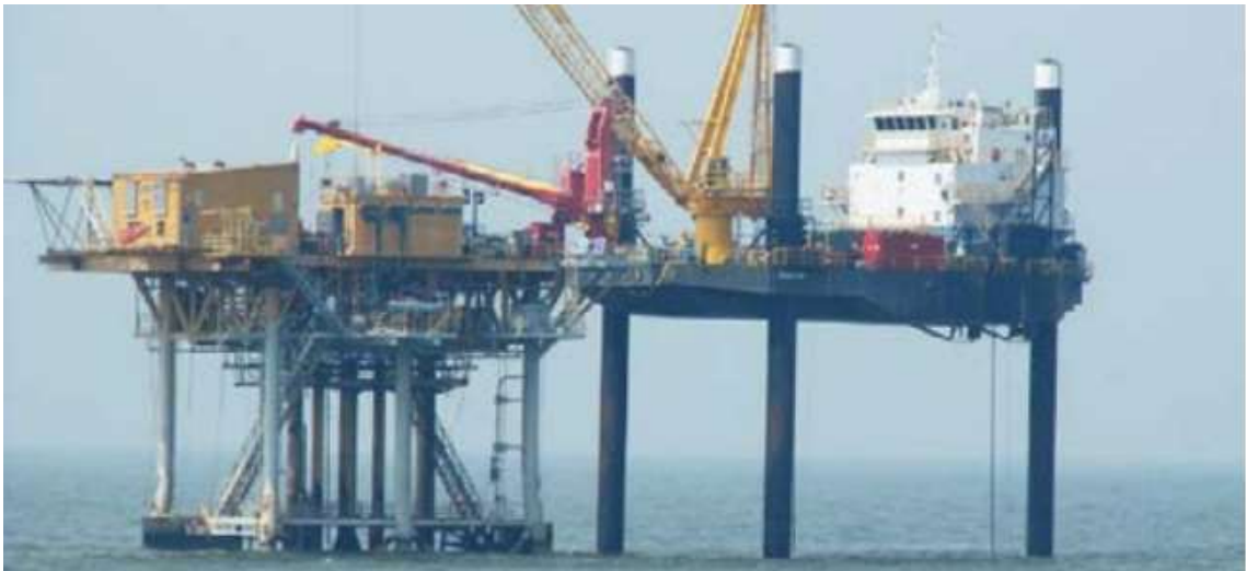
Jack Up Vessel. A jack up rig or self-elevating unit consisting of a buoyant hull fitted with a number of movable legs, capable of raising the hull over the sea surface. This allows transportation of the unit and all attached machinery to a desired location. Once the vessel is in place, it jacks its legs up to the required elevation above the sea surface supported by the sea bed. These are generally suitable for operations in depths of up to 40 metres.
