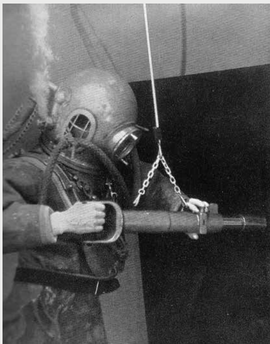
A diver using a Cox Submarine Bolt Driving & Punching Gun. Photo: Temple Cox Development Co. Ltd.
