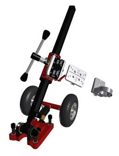
To the four  $40^+$  och  $50^+$  drill stands with universal motor mounting also have Weka and  $\emptyset$  60 mm mounting plates as accessories.
