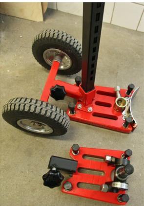
Horizontal and vertical core drilling using 40<sup>+</sup> drill stand
