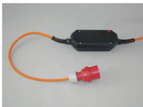
The DK 52 is switched by a double press key assembled in the terminal case on the top of the machine. The main current is as well switched by a contactor assembled into a separate plug-resp. contactor case. By this device the motor is switched solid and exactly as well as an under voltage trip according EN 60 204 is realized.
