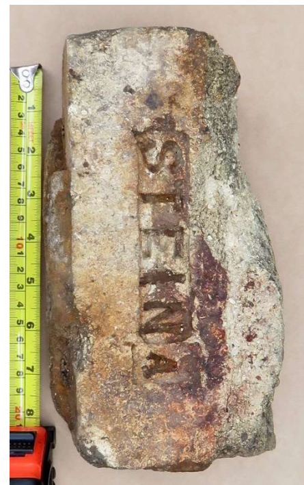
Illustration 20: "Stein A" fire brick: Point G (21 st September 2015)
