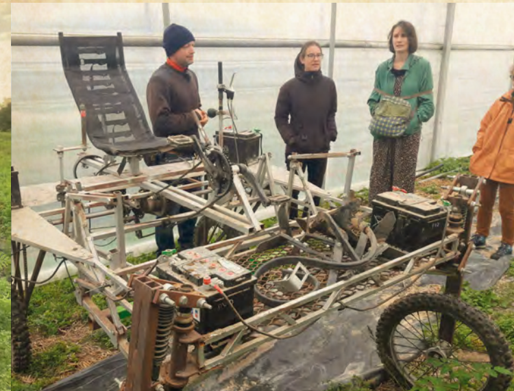
Aggrozouk: pedal-powered tool holders with electric assistance. Self-built equipment by Boris Canal, vegetable farmer, with l'Atelier Paysan. BAG visit in France, 2021.
