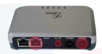
Once we have rebooted the VoIP adapter, we have to **check** that the **cables** are connected correctly. (as shown in image) Internet cable connected to the port **WAN**, the telephone cable connected to **Phone 1** and make sure the **power is correctly connected**
