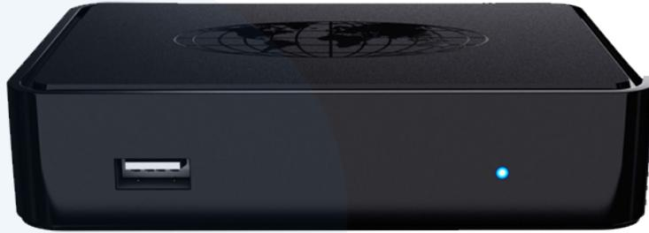
First we have to check that the IPTV BOX has a **blue light** and that its connected to the power.
