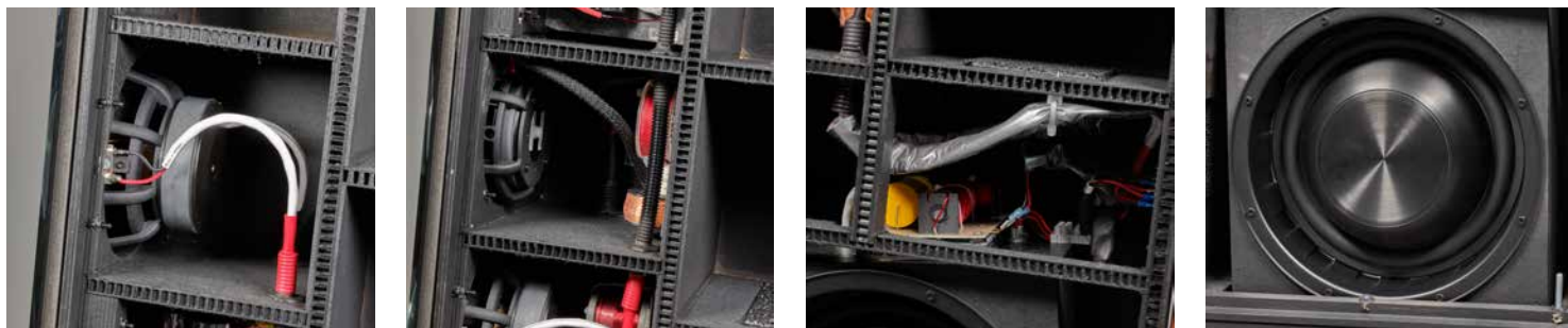
Each chamber of the pattern is a small window into Manfred Diestertich's wondrous world of loudspeaker construction. From left to right: two signal lines to the motor system of one of the woofers – one for the drive and one for the damping coil; the basket of the midrange driver without a centering spider in a flat design; parts of the "floating" crossover with filter elements on both sides of the driver and one of the two 28 cm woofers.
