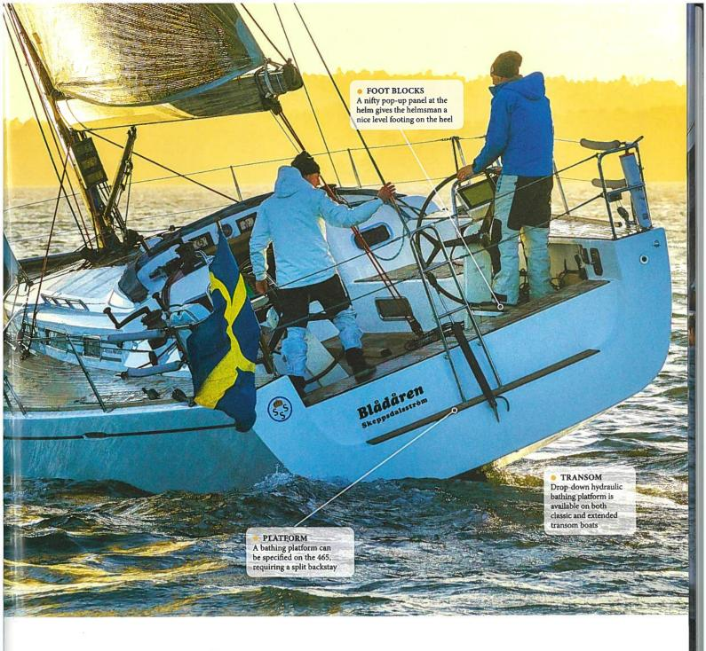
the two wheels which makes it comfortable to stand on even on quite a heel. In lighter airs, a more comfortable position would have been sitting on the quarter, back pressed into the padded guardwires and feet nicely chocked. From here, the helmsman could easily reach the German mainsheet on manual winches just ahead on the coaming. The mainsheet track is recessed into the cockpit just ahead of the pedestals, and we found it easier to spill wind in the gusts using the traveller itself.
