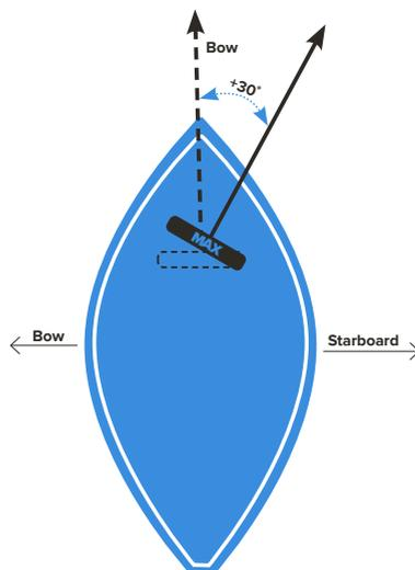
3. Press Save. MAX is now configured for this mounting position and will remember it. Attitude outputs (Heel, Pitch, Compass) will be referenced to the boat and not to MAX. These numbers might not make sense when MAX is not mounted.
