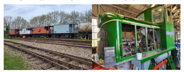
Ketton No3, thanks to Thomas, Alex, George and Gary has moved on to the point where it is near becoming a running locomotive. Much of the bodywork is complete and painted and the engine has been started. It even has operating brakes!
