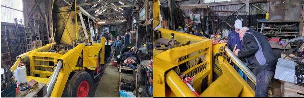
Just outside the Woolsthorpe Shed, Mr. D has been undergoing some major mechanical work to bring her back into service. The transmission has been removed, rebuilt and reinstalled which was no mean feat! Mr. D should be back in operation in which will be a welcomed addition to the operational fleet.
