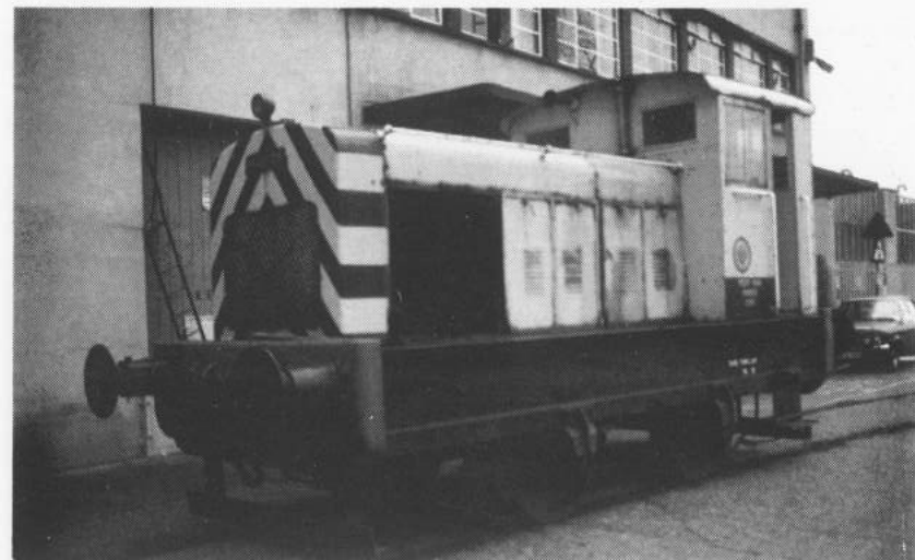
(12) Ruston and Hornsby Class 88DS 4-wheel Diesel Mechanical
