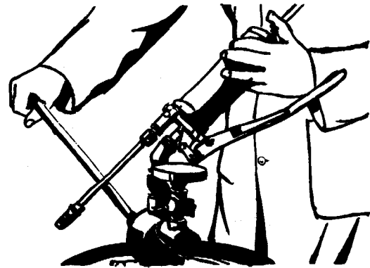
Fig. 6. Using Gun Filler Attachment.
