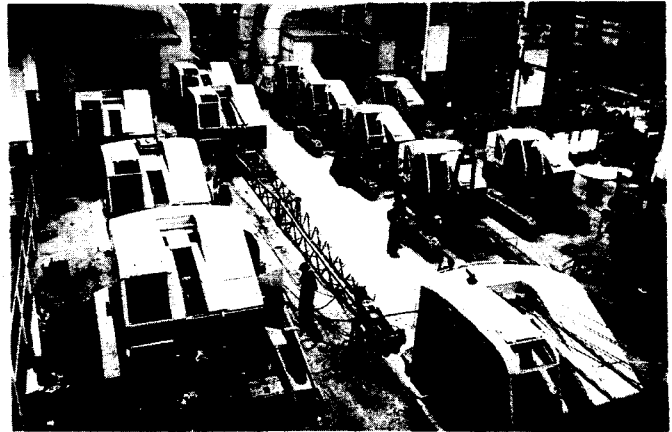
Continuous assembly - lines for smaller excavators (Final stages of Erection).
