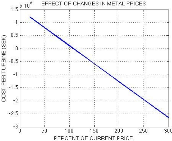
Figure 11 The effect of changing metal prices on economic consequences of decommissioning for a land-based Vestas V82 1.65 MW turbine. The figure shows the full-scope scenario.
