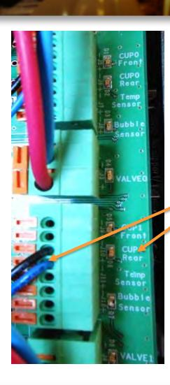
IT IS IMPORTANT TO CONNECT THE CUP SENSOR TO <u>CUP REAR</u> AND NOT TO CUP FRONT!
