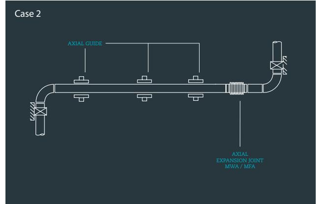
The main anchors are located where pipes change directions in order to consider the straight section as an individual section of piping taking us to case no. 1.
