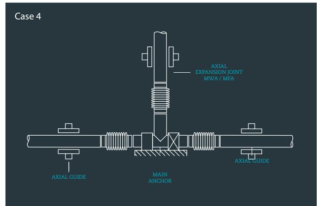
In this case the main fixed point is situated at the intersection where two sections of piping meet.
