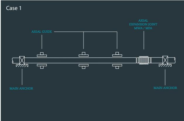
The classic case of an Expansion Joint located in a straight section of piping installed between two main anchors.
