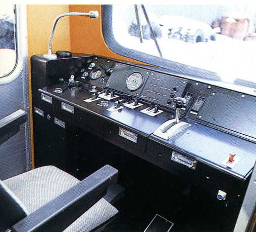
Driver's stand for manual train-control at either end of train unit.
