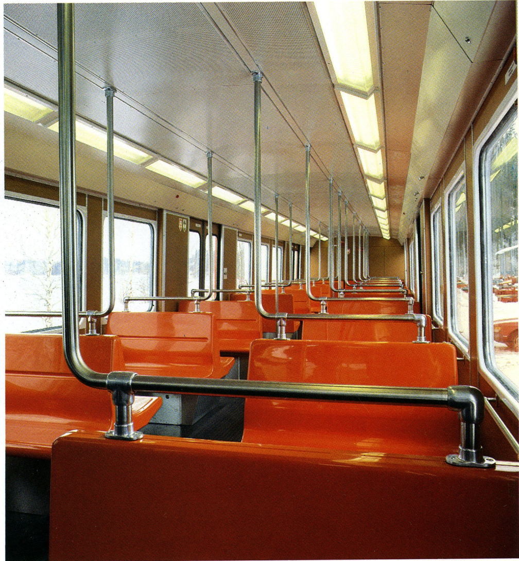
Car with seats of hard, reinforced plastics. Route maps above doors and on surface of lamps in two rows.
