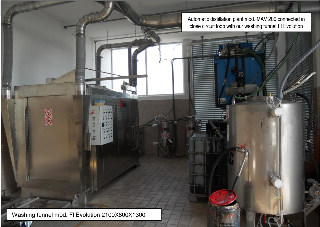
Special device for the washing of no. 08 cylinders (4 Anilox- 4 rubber)
