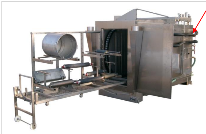
FL EVOLUTION 2100 x 650 x 1100 ALRS manufactured in 2005 Suitable to the washing of the components of the printing presses and ink injection hoses
