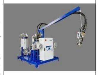
The installation of optional modulating nozzles will, in addition to providing automatic self-adjustment of pouring pressures, also permit the recycle of chemical components through the mixing head at a preset lower output, thus avoiding sudden pressure peaks.
