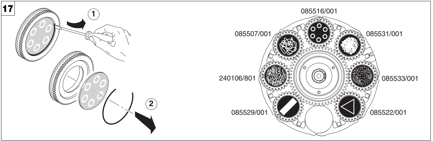
Replacing rotating gobos (ø 25.7 mm - max 23 mm image – thickness max 1.1 mm) - Fig. 17
