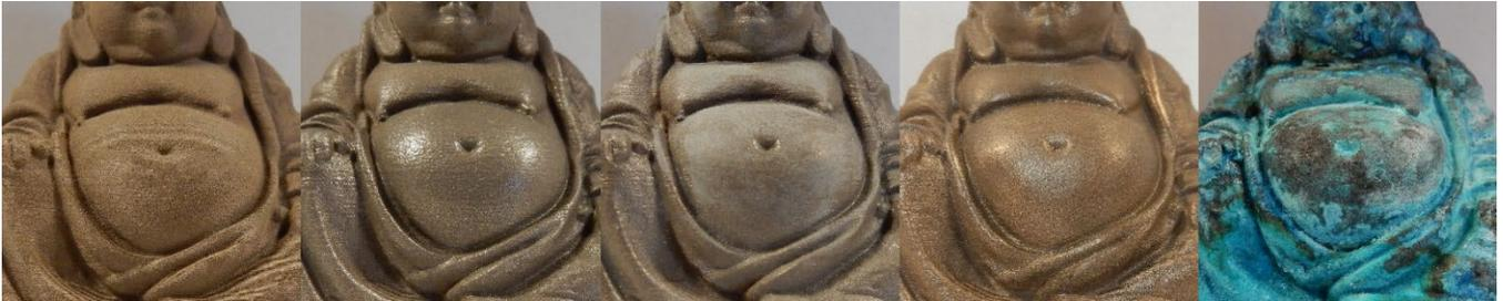
Post-processing the MT range is quite an easy process though manual labour is required when you do not have access to a so called “rock tumbler” which gives the best polished results.
