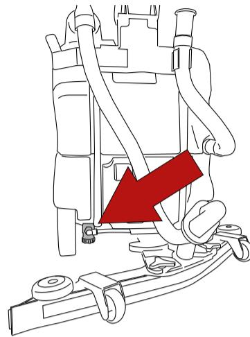
Check that the detergent outlet filter is clean.
