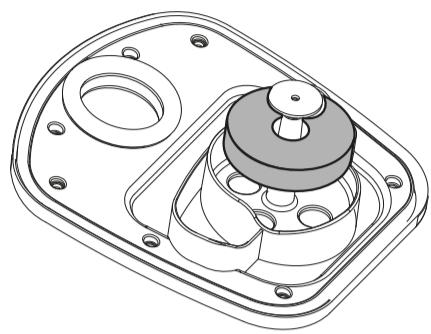
Check the dirty water tank float is undamaged and clean and moves freely on the pin.
