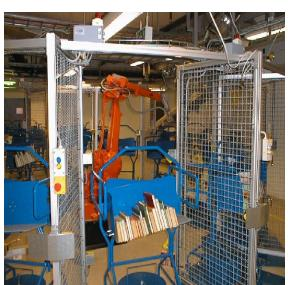
6. Automatic robot in basement for separation of discharged material to various departments.
