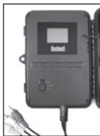
Cable from "A/V Out"
