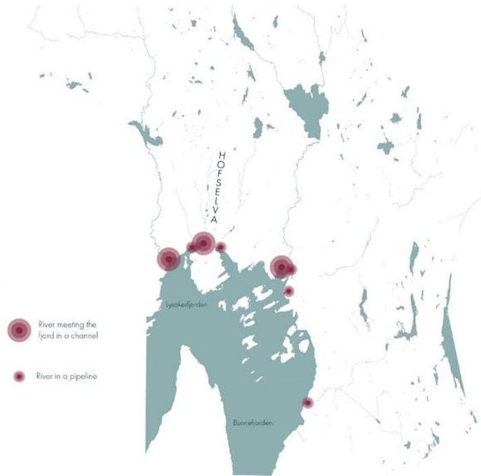
Figure 2: Map showing existing outlets of rivers in inner Oslofjord. Size of icon is indicating whether the outlets are in channels (big circle) or in pipes (small circle).
