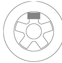
If OPPOSITE POSITION is enabled, the application position for the bottom weight is also indicated on the phase display (6 o'clock) to facilitate cleaning the rim and the relative application of adhesive weights. The symbol used is:
