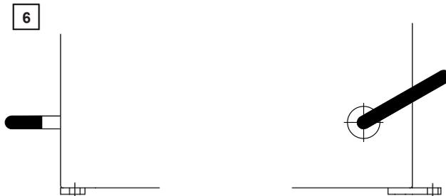
This pedal allows releasing the device fastening the wheel on the adapter. **Do not actuate this pedal during the machine cycle and/or when adapters other than the standard cone adapter are mounted. The pedal has two stable positions: top, wheel unclamped; bottom, wheel clamped.**
