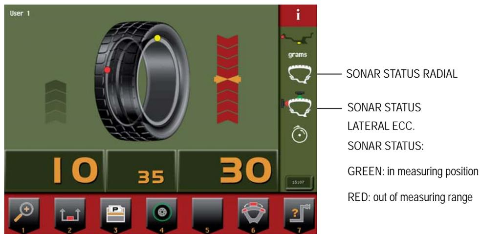
After performing a balancing run, the out-of-balance values are displayed as well as arrows useful for positioning the correction weight at the application point. After positioning and locking the wheel, apply the weight vertically at the top. When the beep signal is enabled (👉 **ACOUSTIC SIGNAL**), reaching of the correction position is accompanied by a “beep”.
