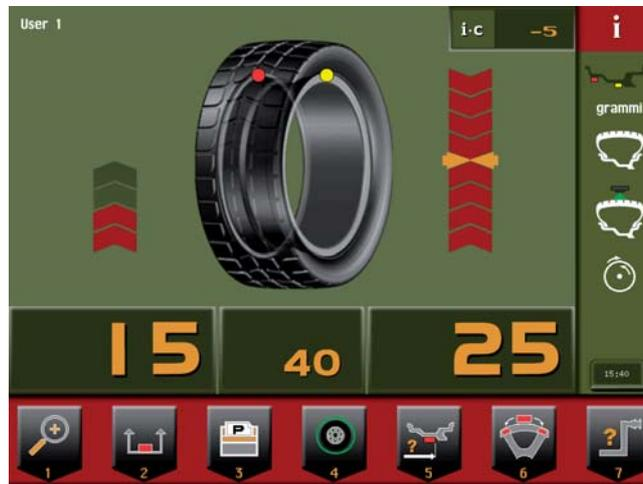
If a special icon appears near the button **5**, it means that the wheel balancer is suggesting static balancing, however, such that also the dynamic torque unbalance will be brought within tolerance.
