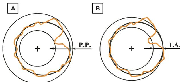
The radial and lateral eccentricity measurements are automatically carried out after the unbalance measurement without having to go into particular procedures. Remember to position the sonar sensors in front of the surface to be
