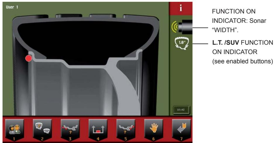
The screen appears upon removing the distance + diameter gauge.
