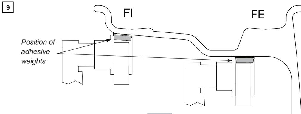
After having detected the dimensions, use the **3** key to indicate the type of correction selected for the inner side.
