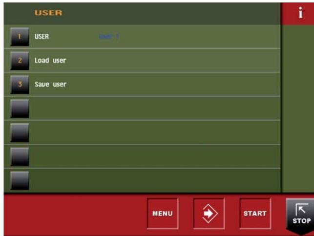
The wheel balancing machine can be used simultaneously by 4 different users who, through a simple sequence, can memorize their work condition and call it when needed. The names of the users can be stored (
