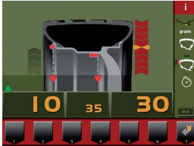
It is recommended always to use this function when correcting the out-of-balance with adhesive weights ALUS. Remember to thoroughly clean the application areas.
