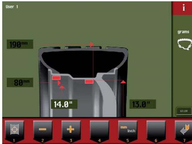
Even in correction mode with adhesive weights, the dimensions can be input or modified manually using the buttons shown on screen in accordance with the technical data displayed.
