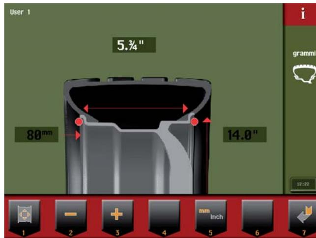
If necessary, the dimensions can be input or edited in manual mode as follows:
