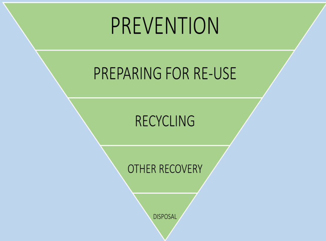
Figure 2: The Waste Hierarchy in the EU Waste Framework Directive, made by One Planet, feel free to use and reuse the figure.
