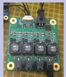
Integrated 4 channel individually controlled LED illumination system
