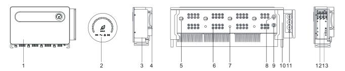
(5)DC switch (1)Front panel (2)LED indicator (4)Support frame (3)Junction box (10)Anti-collision angle (8)USB port (9)COM port (6)PV terminal (7)Vent valve (11)Waterproof silicone pad (12)AC terminal block (13) Grounding copper bar
