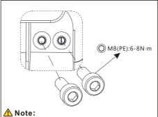
The built-in grounding copper bar is only used as ar equipotential connection point for the protective ground. It cannot be used as a substitute for the protective grounding point of the inverter housing.
