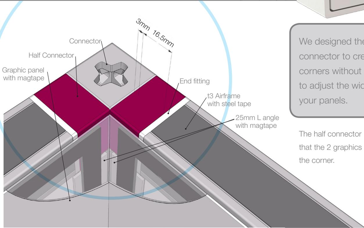
We designed the half connector to create internal corners without having to adjust the width of your panels.
