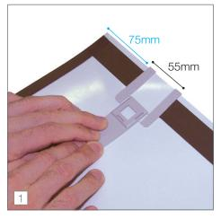
1 When preparing the graphic panel, leave a 55mm gap in the magnetic tape, 75mm in from each side.
