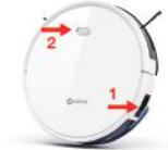
3.4 Switch on the robot vacuum cleaner. Press button (1). Hold down button (2) for 5 seconds.
