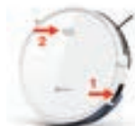
3.4 Switch on the robot vacuum cleaner. Press button (1). Hold down button (2) for 5 seconds.
