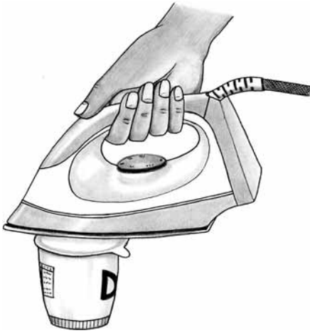
Figure 34: Sealing foil lids with a domestic iron
