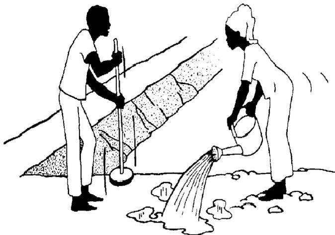
*Figura 13: Compactando o dique (Viveen et al., 1985)*
