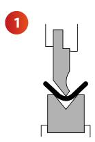
**1. Air bending:** where the sheet metal being bent with the punch does not reach the very bottom of the die. This enables different bending angles to be obtained using the same tools, which requires extreme precision to guarantee a perfect result.
