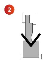
**2. Bottoming:** the punch forces the sheet metal to the very bottom of the die. The bending angle obtained depends on the tools used.
