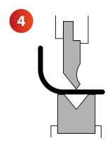
**4. Roller pressing:** this enables different curve radii to be obtained in a sheet by means of subjecting it to multiple bending sequences.
