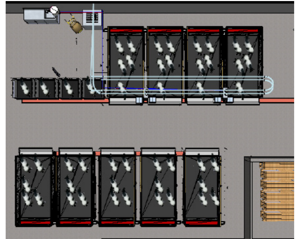
Calf barn with 4 Singleboxes, 4 Groupboxes with Calf Feeder and 5 Groupboxes for weaned calves up to 4-5 months of age. Spacious areas for feeding and bedding material storage. Total area 14 x 18 meters with 49 calf places.
