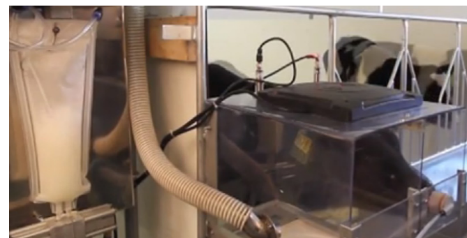
Moving Floor Calf Feeder gives the calves both milk and concentrate.
