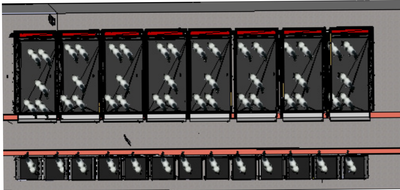
Calf section with 13 Singleboxes and 8 Groupboxes. The area is 21 x 10 meters with 53 calf places.
