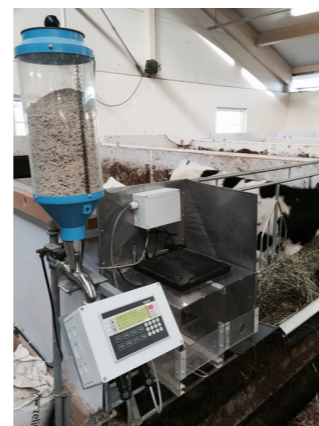
Installation of automatic concentrate feeding.
