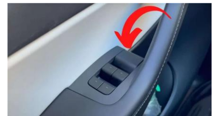
The emergency door opening lever for the Model X front doors is located behind the window control buttons
