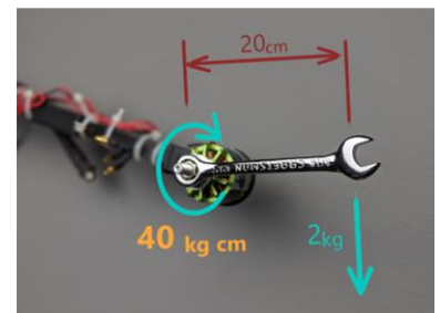
An example of torque is seen when you use a wrench to affix a nut. If you have a wrench that is 20 cm long, and you push down on the wrench with 2 kg of force, the torque on the nut is (20 cm x 2 kg =) 40 kg cm. (Source: https://maker.pro/custom/tutorial/what-is-torque-and-why-does-it-matter )
