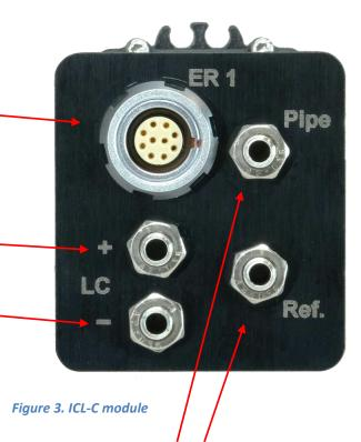
Terminal "**Pipe**" – Pipe/structure connection Terminal "**Ref.**" – Reference Electrode connection
