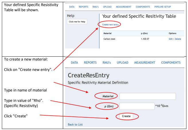
The new material will now appear in "Your defined Specific Resistivity Table" ready to be used when defining an LCS sensor certificate, see "Figure 6." Edit a LCS certificate" page for typing in a value for DC resistance."
