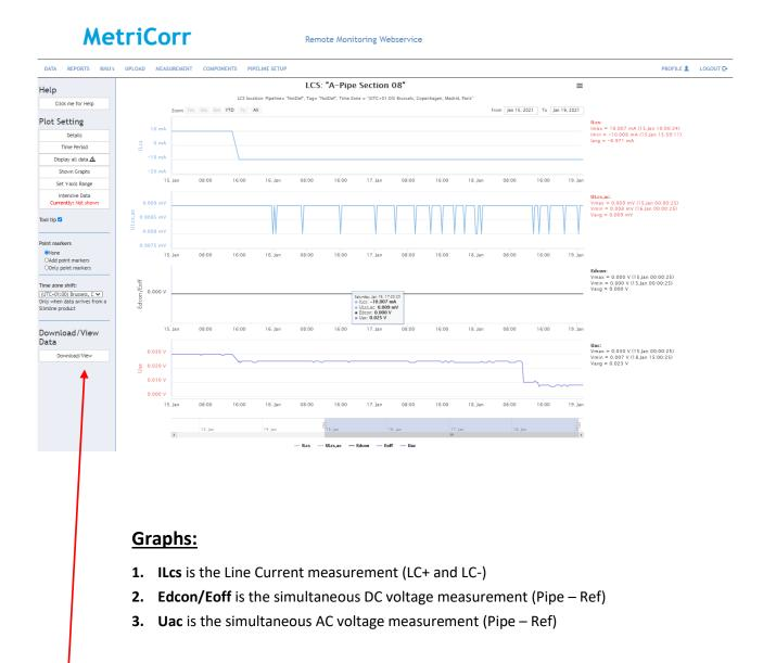
Click "Download/View Data" to view a list of each measurement, including the (Line Current AC voltage measurement, ULcs, ac), illustrated on next page.
