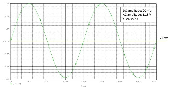
If the LC input voltage exceeds 1.2 V, the A/D converter will clip the signal and an error message will be shown.
