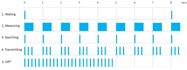
\*The device is Off. 5 short (0.5 milliseconds) flashes per second for 5 seconds. This signal is triggered by a **short** (<0.5s) push on the pushbutton. Figure 4. LED flash indication
