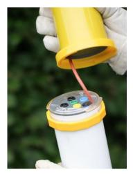
The MetriCorr Big Fink Battery requires only that power cord connected to connector E (Figure 2), as per **step 3** above. Once power is connected, ensure that the logger is ON and set up correctly (**see Section 3**).
