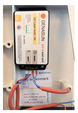
Step 5: Connect the Solar Charger to the solar panel
