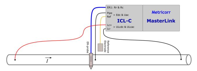
The current "I" with an arrow indicates the positive current direction.
