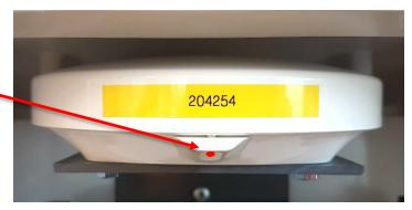
operate. When the relay is switched off, the modem will stay on (indicated by the red LED) for a while until the super capacitor has been discharged.
