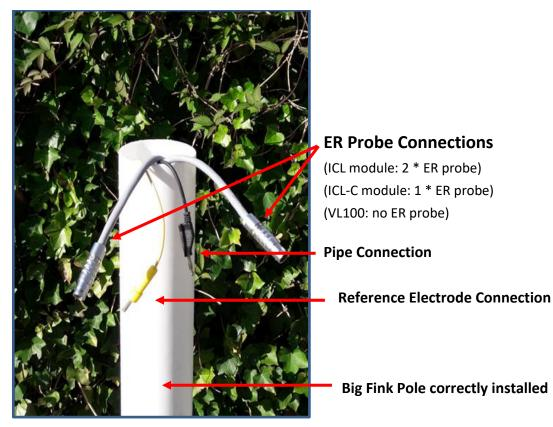
Figure 11: Big Fink Test Station ready for installation of Slimline series: "ICL & MasterLink". Note that "ICL-C & MasterLink" only takes one ER probe, Pipe connection (black), Reference (Yellow) and two wires for pipe connections for "LC+" and "LC-".
