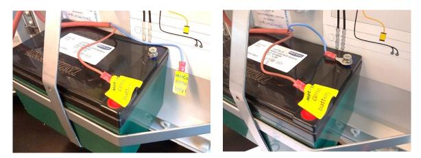
5. Remove yellow tape from the connector (blue wire from solar panel), insert it into the solar panel terminal marked "Panel –" and tighten the screw terminal:
