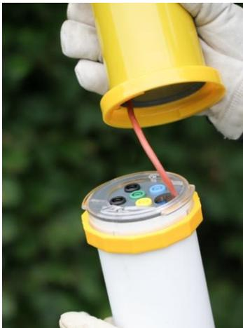
The MetriCorr Big Fink Battery requires only that power cord connected to connector E (Figure 2), as per **step 3** above. Once power is connected, ensure that the logger is ON and set up correctly (**see Section 3**).
