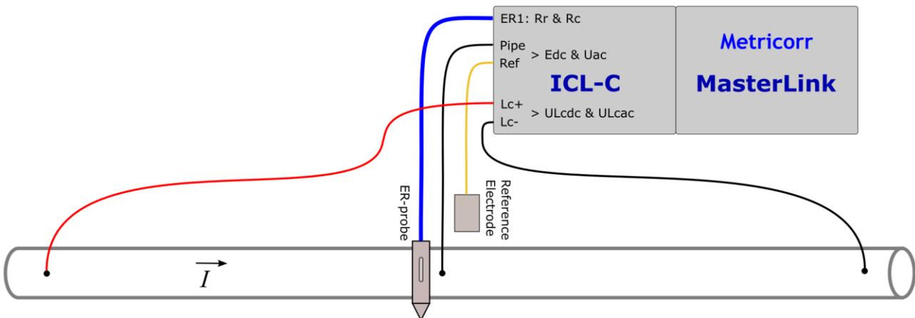
To calculate the DC current flow from the measured Line Current voltage, the DC resistance of the pipe section has to be typed into the app.
