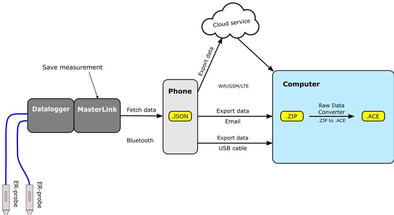
1. The datalogger takes measurements (i.e. once an hour), where the measurement data is stored in the MasterLink.
