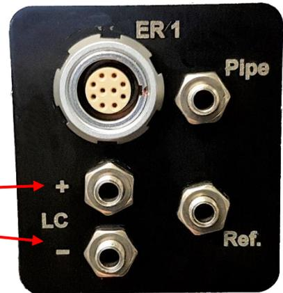
A steel pipe is used for this illustration, where the ICL-C MasterLink is placed in the center between the two line current measuring points (Lc+ and Lc-):
