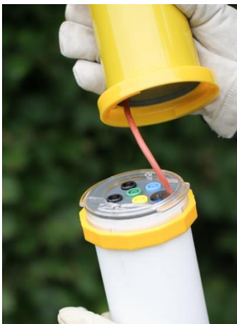
Figure 15: Big Fink Battery Hat General layout & appearance
