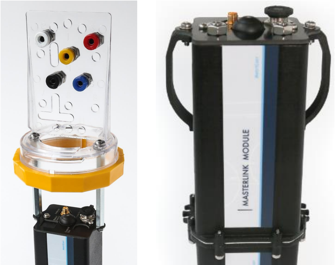
Figure 11: Left: Big Fink terminals. Right: Mounting brackets and Clips for Slimline Installation in Big Finks
