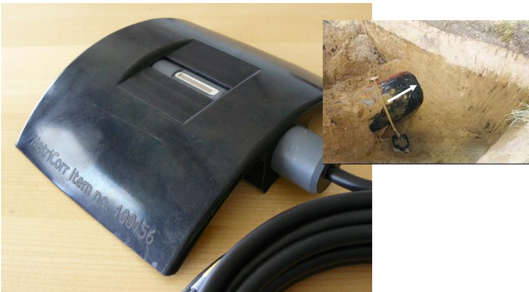
Rod type ER probe embedded in sleeve for providing a better integration with a pipe surface.
